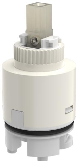
HANSAECO control cartridge 3.5; water brake at approx. 50% water rate; with ceramic discs; adjustable hot water stop; volume restrictor indefinitely variable up to approx. 6 l/min
